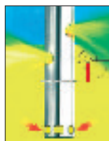
Mixing apertures open: The fluid is being mixed and pumped
